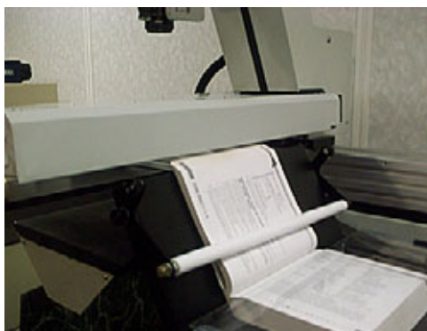
Image 5: 120° option with the glass in a lowered position
